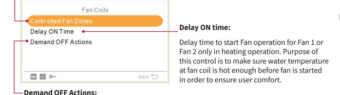
The purpose of this control is to enhance user comfort by allowing to stop fan or keep it in operation when Demand OFF conditions by room temperature are fulfilled.
