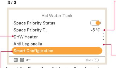
**Smart Configuration:** Option to allow the tank to be heated to an intermediate temperature of comfort in conditions of water consumption in order to avoid heating to the traditional setting temperature (Only available in Economic mode).
