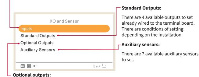
There 4 additional available outputs to set. These 4 additional outputs are not wired to the YUTAKI terminal board.
