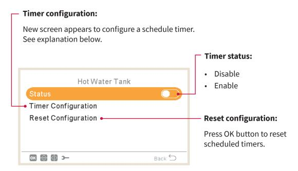
Pressing the OK button with "Timer Configuration" being selected displays the detailed schedule screen. The active schedule timers are shown in a weekly calendar.
