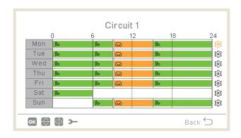
Up to six timer events can be defined for each weekday, and these can be used for turning the operation ON or OFF or operation mode (ECO or Comfort). Pressing the OK key with one of the weekdays being selected in the weekly calendar screen displays the detailed schedule for the weekday.
