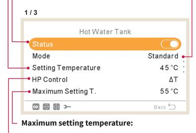
Maximum value of DHW setting temperature permitted by the installer.
