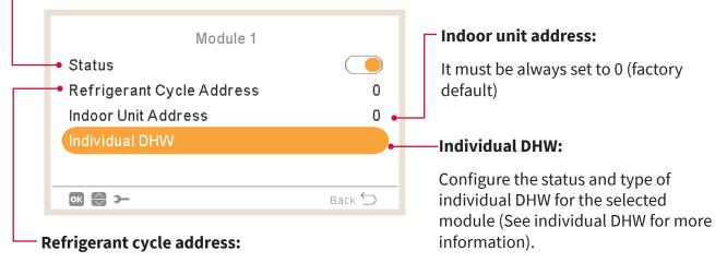
Set the refrigerant cycle address for each module, making sure that the setting is common with that of the outdoor (DSW4-RSW1) and indoor (DSW15 - RSW2) units which are part of the module.
