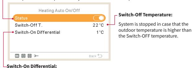
Differential temperature between average outdoor temperature of the previous day and the Switch Off temperature.
