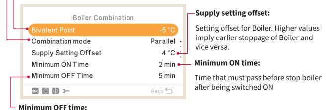
Time that must pass before start boiler after being switched OFF
