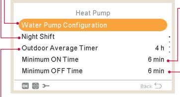
Minimum ON time: In order to reduce a possible compressor damage, demand ON cycles can be reduced by determining the time that must pass before accepting new Demand OFF.
