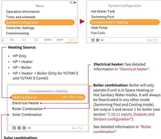
The solar combination will enable you to heat up your domestic water by means of the sun whenever the sun is available.
