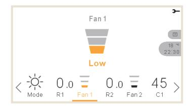
Room 1 or 2 could control Fan Coils. Once configured to control them on the menu, the bottom bar includes the option to manage those fan coils:
