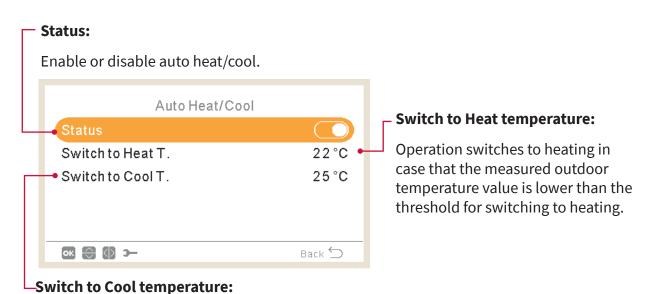
Operation switches to cooling in case that the measured outdoor temperature value is higher than the threshold for switching to cooling.
