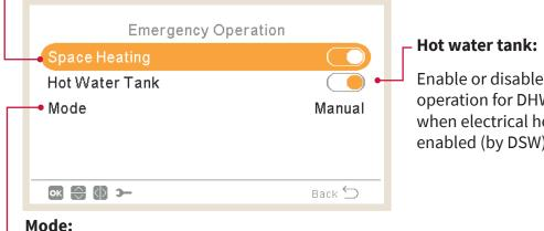
Enable or disable emergency operation for DHW. Only available when electrical heater for DHW is enabled (by DSW).
