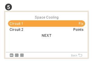
Configure circuit 1 and circuit 2 options (Only available for cooling mode): Deactivated, Points, Gradient, Fix.
