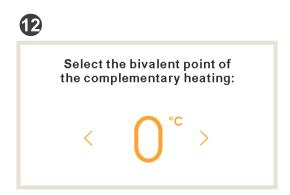
• Select the bivalent point for boiler or electric backup heater (from -20°C to 20°C).
