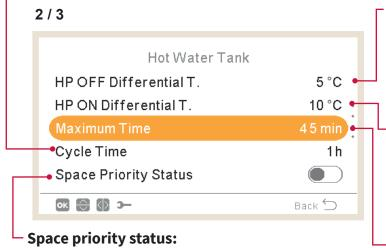
If space priority function is enabled, Heat Pump operation by DHW mode stops (and continue with DHW heater, if necessary).
