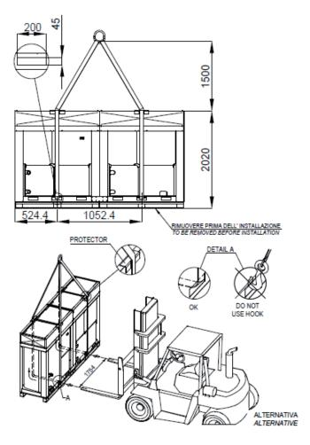
Figure 2 - Lifting the DUAL unit
