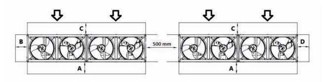
Figure 5 - Units installed side by side along their shorter sides, B or D
