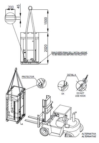
Figure 1 - Lifting the MONO unit
