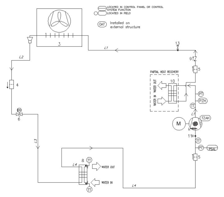
Figure 18 - Refrigerant circuit (P&ID) diagram for MONO circuit EWAT~CZ unit
