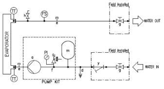
Figure 8 - Hydraulic diagram
