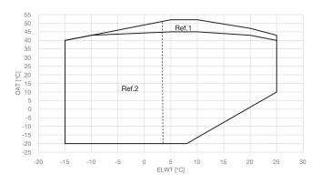
Figure 12 - Operating limits on EWATCZ
