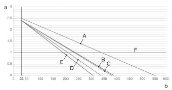
*Figure 16* – Initial expansion vessel pressure on the basis of maximum water volume
