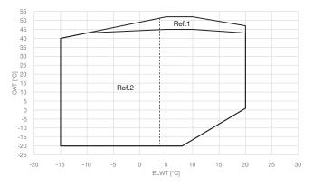
Figure 13 - Operating limits on EWYTCZ in cooling mode
