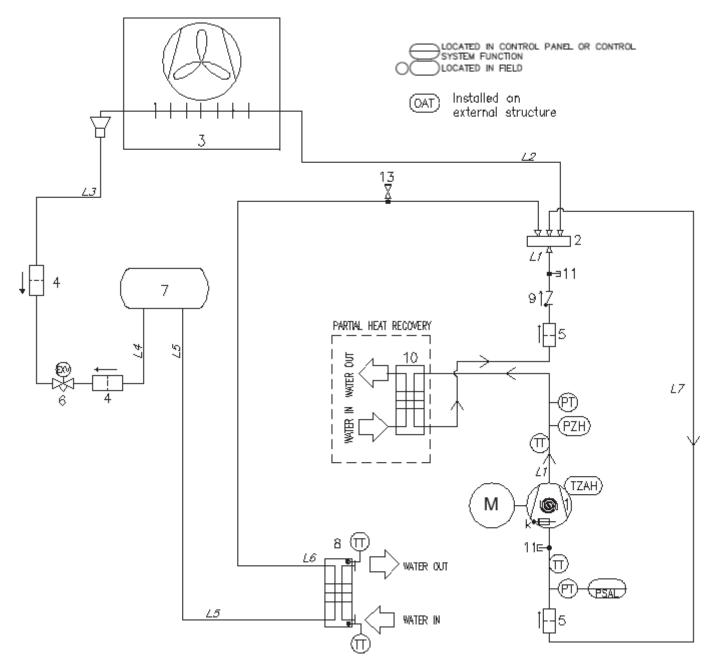
Figure 17 – Refrigerant circuit (P&ID) diagram for MONO circuit EWYT~CZ unit
