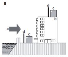
Figure 7 - Seaside installation of the outdoor unit
