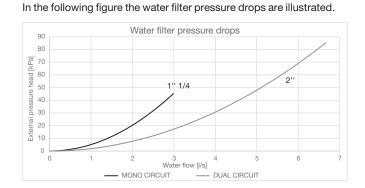
Figure 9 – Water filter pressure drops
