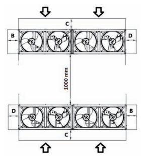
Figure 6 – Units installed side by side along their longer sides (Case 1 and Case 2)
