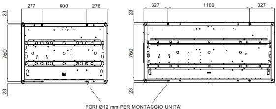
UNIT MOUNTING HOLES Ø12 mm
