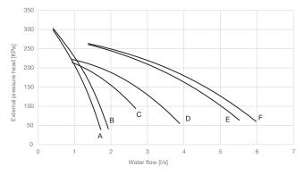
Figure 10 - External pressure head of Low Lift Pump
