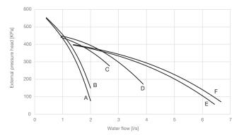
Figure 11 - External pressure head of High Lift Pump
