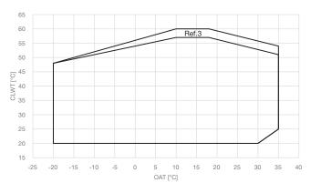
Figure 14 - Operating limits on EWYTCZ in heating mode
