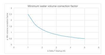
Figure 15 - Minimum water volume correction factor
