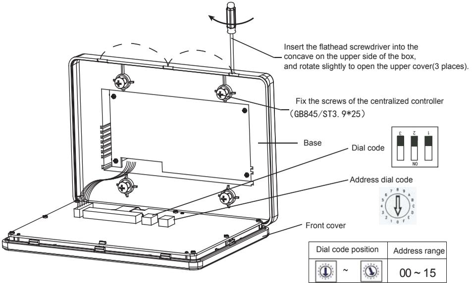
Fig. 1.2 Installation diagram
