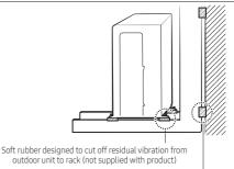
Soft rubber designed to cut off vibration from rack to wall (not supplied with product)
