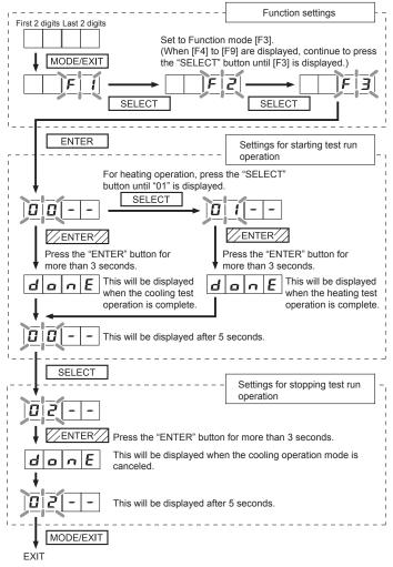
After the test operation is complete, turn off the power. Attach the cover of the electrical component box and the front panel of the outdoor unit.
