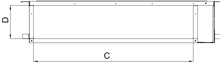
Fig.35 Return Air Inlet
