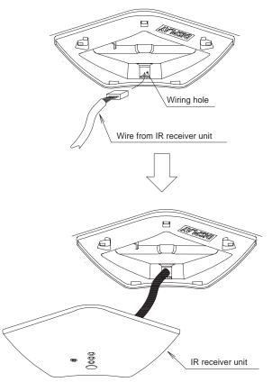
③ Hang the STRAP on the hook of the decoration panel. After that, mount the IR receiver unit onto the decoration panel.
