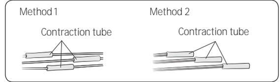
7 After tube contraction work is completed, wrap it with the insulation tape to finish. Three or more layers of insulation are required.
