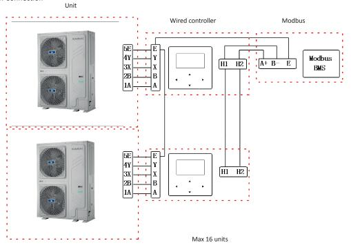
Figure 4-2.7: Wiring
