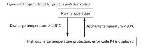
When the discharge temperature rises above 115°C the system displays P4 protection and the unit stops running. When the discharge temperature drops below 90°C, the compressor enters re-start control.
