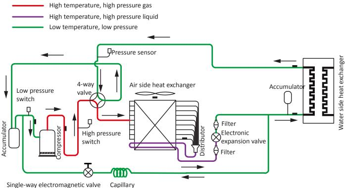
Part 2 - Component Layout and Refrigerant Circuits
