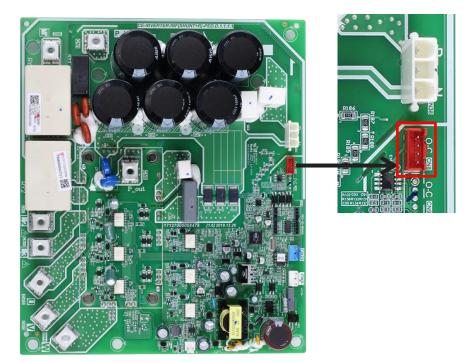
3. When replacing an inverter module, a layer of thermally conductive silica gel should be painted on the IPM module (on the reverse side of the inverter module PCB). Refer to Figure 4-4.3.
