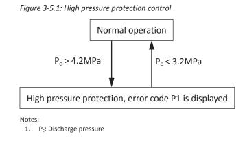
When the discharge pressure rises above 4.2MPa the system displays P1 protection and the unit stops running. When the discharge pressure drops below 3.2MPa, the compressor enters re-start control.
