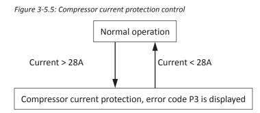
When the compressor current rises above  $Current_{max}$  the system displays P3 protection and the unit stops running. When the compressor current drops below  $Current_{max}$ , the compressor enters re-start control.
