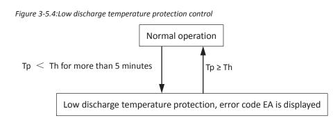
When the discharge temperature is lower than suction temperature for more than 5 minutes, the system displays EA protection and the unit stops running. When the discharge temperature is higher than suction temperature, the compressor enters re-start control.
