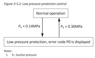
When the suction pressure drops below 0.14MPa the system displays P0 protection and the unit stops running. When the suction pressure rises above 0.3MPa, the compressor enters re-start control.
