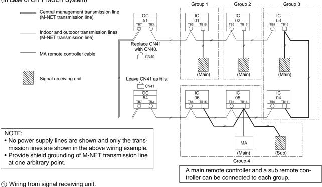
Connected to MA remote controller wiring terminal block (TB15) on the indoor unit. (The terminal block has no polarities.)
