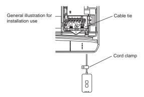
3. Connect the cable to the CN-CNT connector at the indoor unit.
