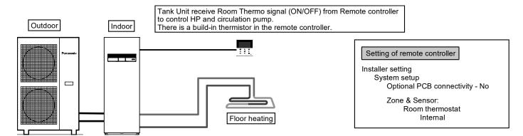
Connect floor heating or radiator directly to the Tank Unit.
