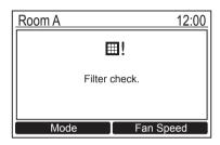
"Filter check" is displayed on the screen if you start running the air conditioner when "
