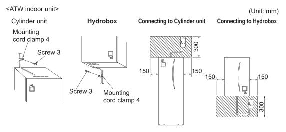
Mount in the same procedure for air conditioner. Please refer to "When mounting on the wall" on 1. Connecting the Wi-Fi interface (1), "Air conditioner".
