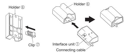
Slip the clip  $\bigcirc$  over the edge of corner box to fix the interface unit  $\bigcirc$ . Note: Mount the interface unit 1 on the side of the indoor unit.
