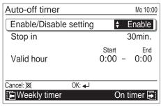
For [Stop in], adjust the timer with the [Cursor button (Up/Down)]. To complete the setting, press the [Enter button].
