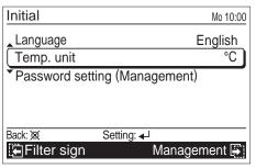
Select [°C] or [°F] with the [Cursor button (Up/Down)] and press the [Enter button].
