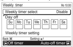
2. Select any of [Weekly 1], [Weekly 2], or [Disable] with the [Cursor button (Up/Down)], and press the [Enter button].
