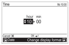
To complete the setting, press the [Enter button]. The screen returns to the "Date and Time" screen.
