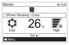
If multiple timers have been set, up/down arrows ▲ ▼ are displayed in the message balloon. To check the target timer function, press the [Cursor button (Up/Down)].
