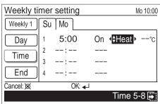
(6) When you selected On timer, adjust the desired temperature with the [Cursor button (Up/Down)].
