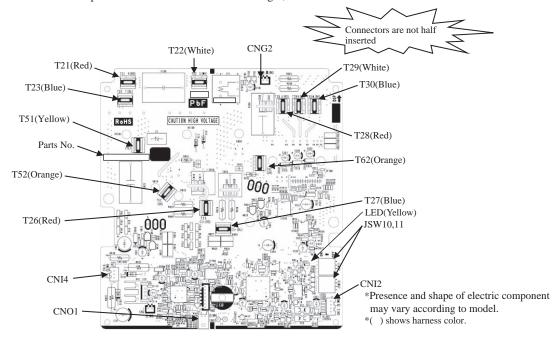
Fig.1Parts arrangement view of inverter PCB
