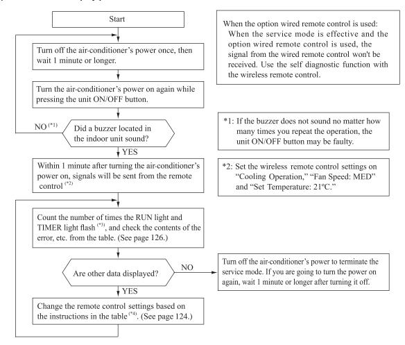
\*3: To count the number of flashes in the service mode, count the number of flashes after the light lights up for 1.5 second initially (start signal). (The time that the light lights up for 1.5 second (start signal) is not counted in the number of flashes.)
