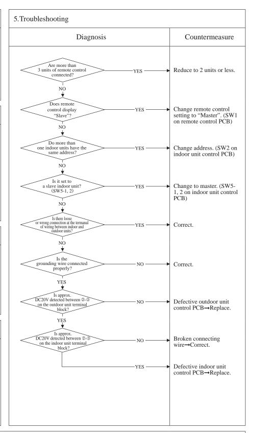
Note: If any error is detected 30 minutes after displaying "WAIT "on the remote control, the display changes to "INSPECT I/U".
