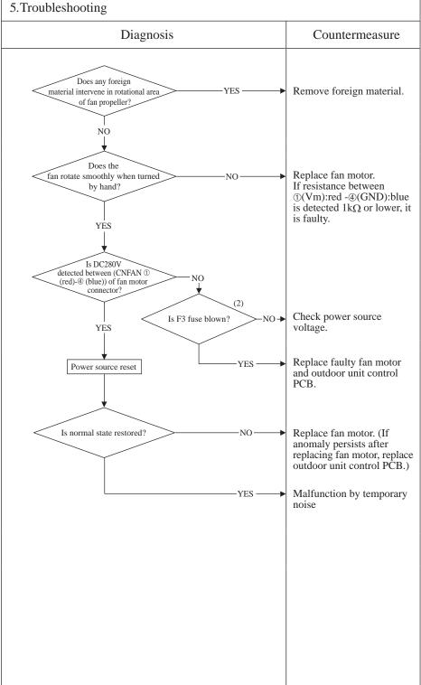
Note: When E48 error occurs, in almost cases F3 fuse (2A) on the outdoor unit control PCB is blown. There are a lot of cases that fuse is blown and E48 occurs due to defective fan motor. And even though only the outdoor unit control PCB ( or fuse) is replaced,, another trouble (\*1) could occur. Therefore when fuse is blown, check whether the fan motor is OK or not.
