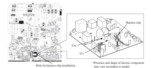
Fig.4 Fix the harness on the harness clip
