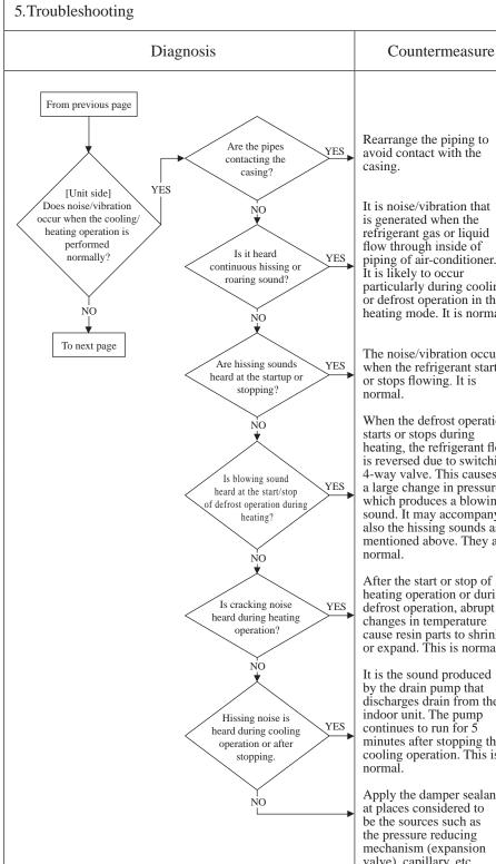
Rearrange the piping to avoid contact with the
