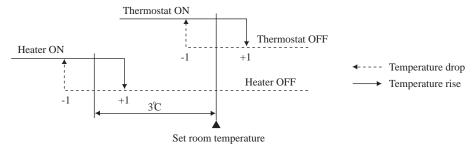
(iii) Thermostat is turned ON when the room temperature is in the range of -1 < Set point < +1 at the start of heating operation (Including from cooling to heating).
