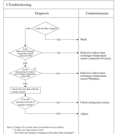
Note: During heating operation; After starting compressor, compressor rotation speed is decreased by detecting indoor heat exchanger temperature (Thi-R) in order to control high pressure.
