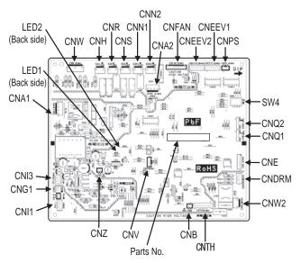
Fig.1 Parts arrangement view
