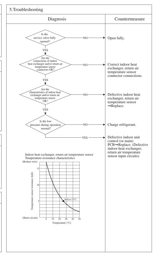
Note: Insufficient refrigerant amount preventive control makes compressor stopped, if it judges insufficient refrigerant amount by detecting the temperature difference between indoor heat exchanger (Thi-R) and return air temperature (Thi-A) for 1 minute after compressor ON in cooling or dehumidifying mode and for 9 minutes after compressor ON in heating mode. [ in cooling mode: (Thi-A)-(Thi-R) \le 4degC, in heating mode: (Thi-R)-(Thi-A) \le 4degC]
