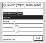
TOP screen Menu ⇒ Energy-saving setting ⇒ Infrared sensor control or Motion sensor control
