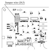
Notes: (1) Default states of the jumper wire (JA3) and the interface kit at the shipping from factory –On the PCB, the DIP switch (SW2-4) is set to enable the annual cooling function.
