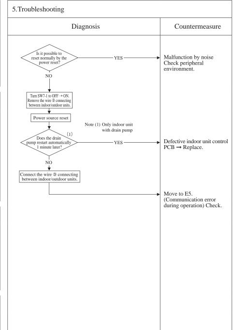
Note: If the indoor unit cannot communicate normally with the remote control for 180 seconds, the indoor unit PCB starts to reset automatically.
