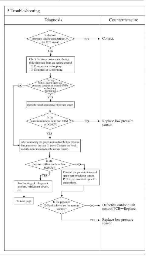
Note: \* Connect the gauge manifold to the service valve check joint during cooling, or connect it to the check joint at internal piping of outdoor unit during heating.
