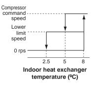
Notes (1) When the indoor heat exchanger temperature is in the range of 2.5-5°C, the speed is reduced by 4 rps at each 20 seconds.
