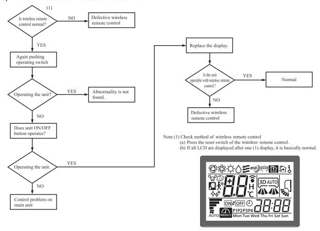
Simplified check methd of wireless remote control It is normal if the signal transmission section of the wireless remote control emits a whitish light at each transmission on the monitor of digital camera.
