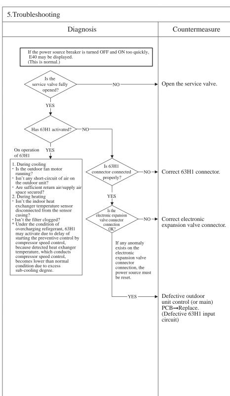
Note: In the protective control range for compressor startup (initial startup after power ON), even if 63H1 is activated only once (63H1turns OFF), immediately the error is displayed.
