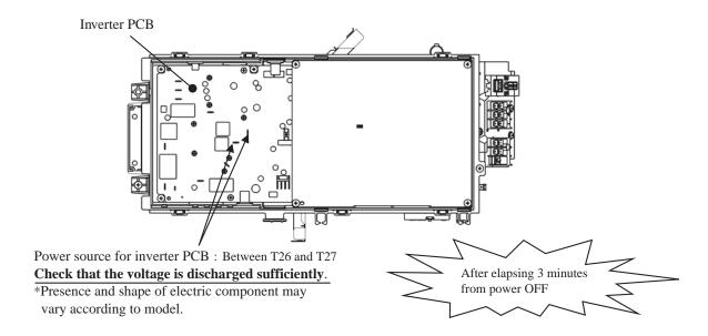
Fig.2 Voltage measurement points
