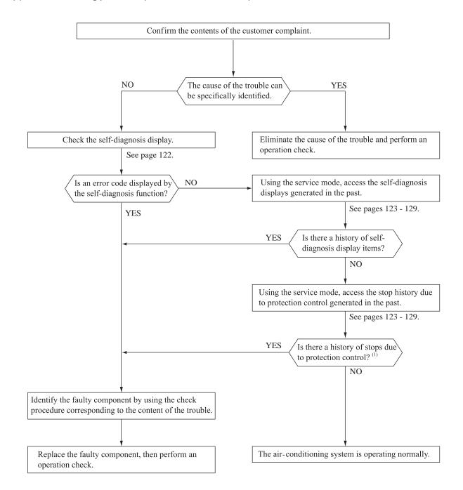
Note (1) Even in cases where only intermittent stop data are generated, the air-conditioning system is normal. However, if the same protective operation recurs repeatedly (3 or more times), it will lead to customer complaints. Judge the conditions in comparison with the contents of the complaints.
