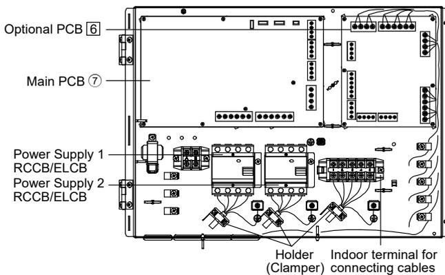
How to guide the optional cables and power supply cord
