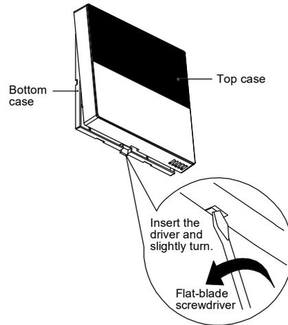
3. Reverse the steps 1 to 4 of section "Remove The Remote Controller From Tank Unit" to fix Remote Controller Case [4] on Tank Unit.
