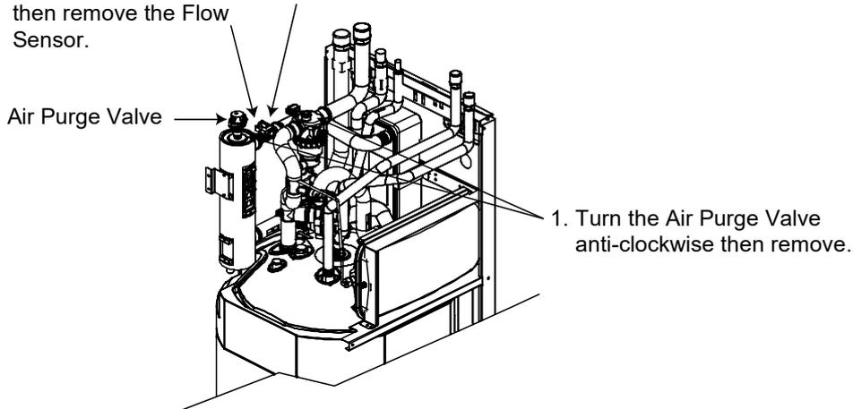
⚠ When reinstall Flow Switch, ensure the arrow on the flow switch is parallel with the pipe shaft and is facing in the direction of flow.
