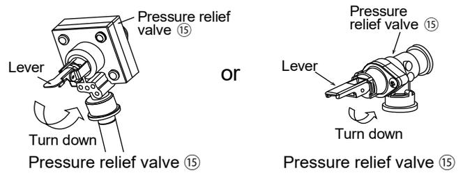
3. Start filling water (with pressure more than 0.1 MPa (1 bar)) to the Space Heating / Cooling circuit via Tube Connector (a). Stop filling water if the free water flow through Pressure Relief Valve (15) drainage hose.
