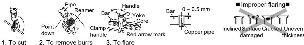
When properly flared, the internal surface of the flare will evenly shine and be of even thickness. Since the flare part comes into contact with the connections, carefully check the flare finish.
