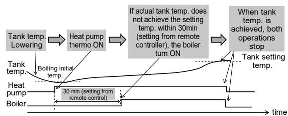
In Advanced Parallel mode, setting for both heating and tank can be made simultaneously. During operation of "Heating/Tank" mode, when each time the mode is switched, the boiler output will be reset to OFF. Please have good understanding on the boiler control characteristic in order to select the optimal setting for the system.
