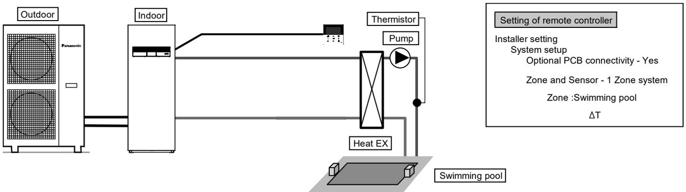
This is an application that connects to the swimming pool only. Connects pool heat exchanger directly to Tank Unit without using buffer tank. Install pool pump and pool sensor (specified by Panasonic) at secondary side of the pool heat exchanger. Remove remote controller from Tank Unit and install in room where floor heating is installed. Temperature of swimming pool can be set independently. This system requires the Optional PCB (CZ-NS5P).
