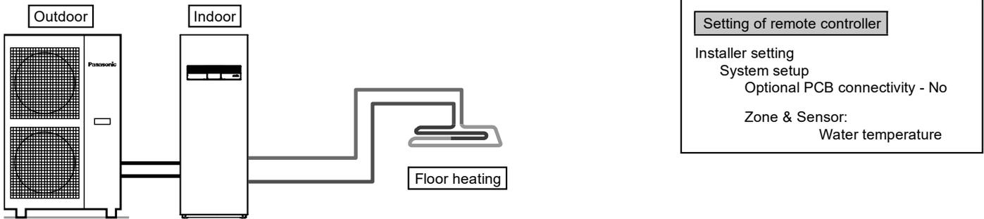
Connect floor heating or radiator directly to the Tank Unit.
