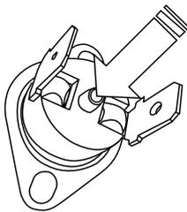
Use test pen to push this button for reset Overload protector ⑫.
