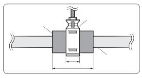
Insulate the gas side and liquid side pipe, noting the
