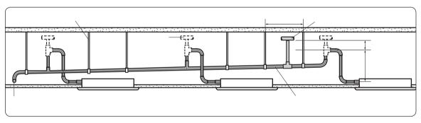
If 3 or more units are installed, install the main air vent at the front of the farthest indoor unit from the main drain
