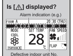
If any of the following alarm indications appears, stop operation once and restart approx. 1 minute later. (Alarm indication, off) [•E04 •E06 •P10 •P20 •H06]
