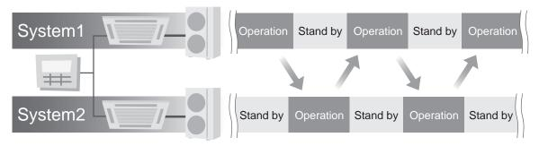
The rotation operation can be set only when controlling 2 refrigerant systems of Single split system (combination of 1 outdoor unit and 1 indoor unit) by one remote controller.
