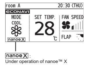
nanoe™ X For a freshness and cleaner environment nanoe™ X generates negative ions using the air in the room to give a healthy air. It also reduces the smell in the room, and constrains propagations of mold and bacteria.
